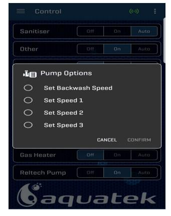
• Sanitisation: Option to utilise a Dosing system during Heating but outside of Filtration Times. Normally, sanitisation via dosing will occur only during the set filtration times. However, the filtration pump may continue to run for extended periods outside of the filtration times due to the pool being heated via either a gas heater, electric heat pump, or solar heating. Utilising this option will allow the continuation of dosing during these extended heating times.
