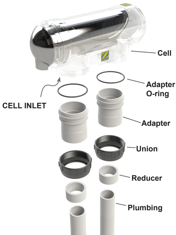
Figure 5. Cell Plumbing Assembly
